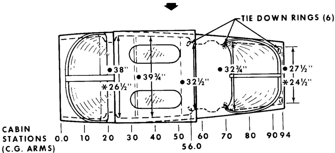
Figure 6-5. Internal Cabin Dimensions
